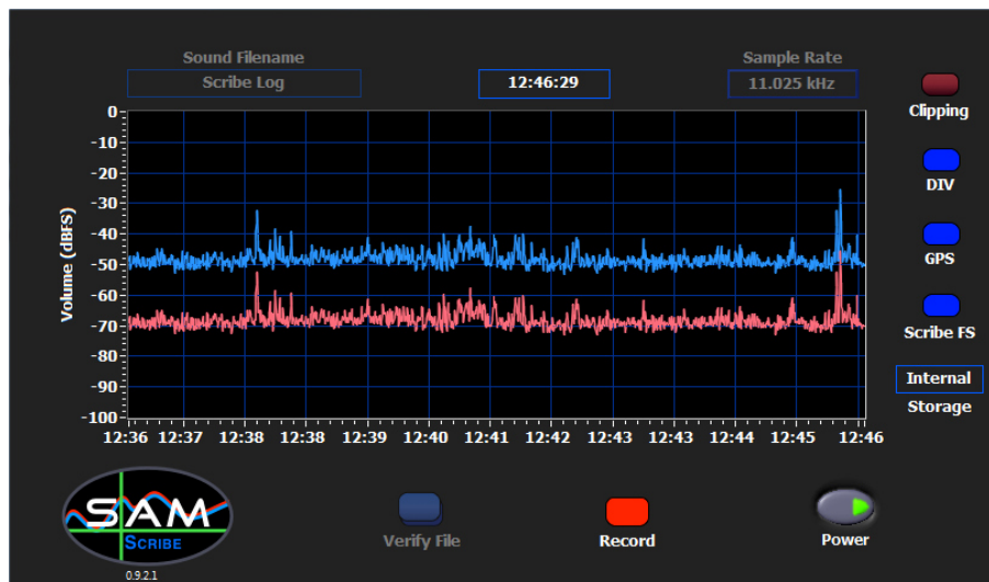
Figure 2: Screenshot of the SAM Scribe recording software. The base name for the recordings is entered at the top right. The sampling rate is chosen at the top right. The other inputs are at the bottom. All indicators are at the right of the screen.
