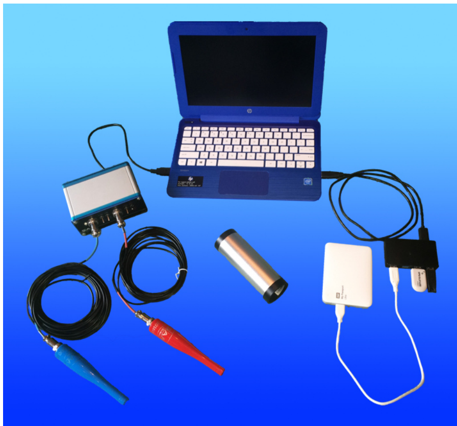
Figure 1: Main components of the SAM Scribe recording system (Mk 1 version). The SAM Scribe FS unit is shown on the left, with the microphones below and the notebook computer in the centre, top. The calibrator is shown in the centre. The USB hub at the right has an external hard drive (left), a GPS (centre) and the security hasp (right) attached.
